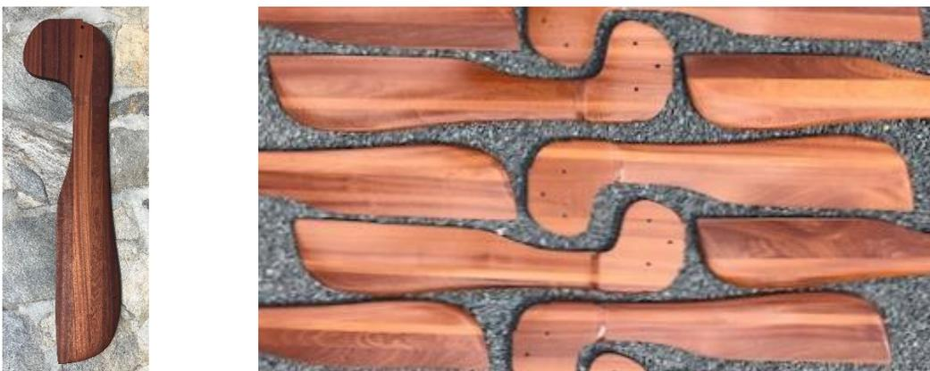
*Above: first production FS rudder blades, provided with holes for quick replacement in the standard attachment hardware.*
