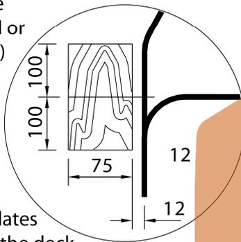
Wooden backing plates are under the deck for the fitting of cam or clam cleats
