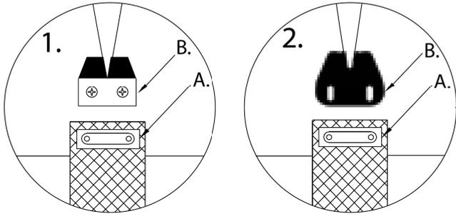
Mainsheet block shall be attached to eyestraps in position A.
