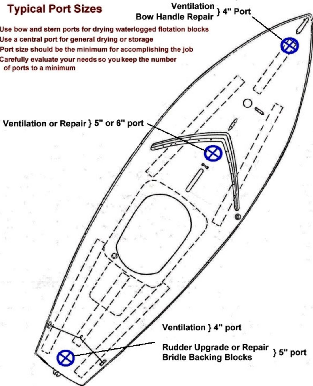
Installing an inspection port is relatively simple. It requires basic tools and materials and can usually be successfully accomplished by someone with a minimum of experience with either.
